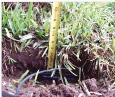
Fig. 3: The Baseline Watertec S100 soil moisture sensor was buried in a trench at a 6 inch depth chosen by the irrigation contractor.
